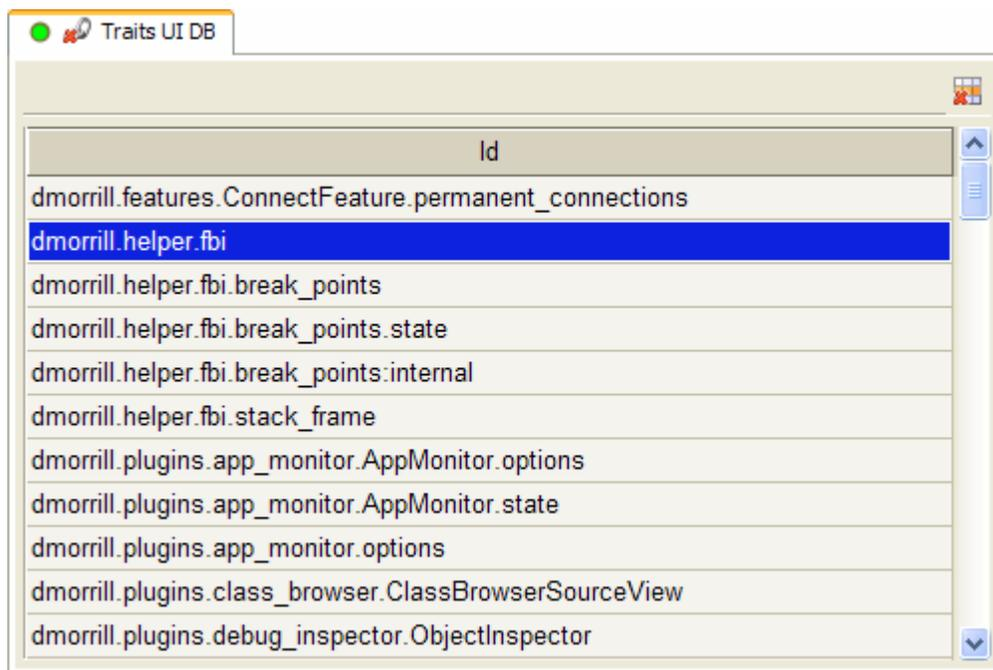
The tool lists the IDs of all current Traits UI database entries in alphabetical order. To delete an ID and its associated data from the database, select the ID and clicking the delete icon (🗑️) that appears on the top-right hand side of the list.
