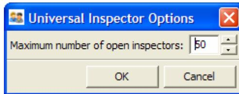
Change **Maximum number of open inspectors** to the value you want, and then click **OK**. If the new value is smaller than the current number of open inspectors, the oldest items in excess of the new maximum are deleted.
