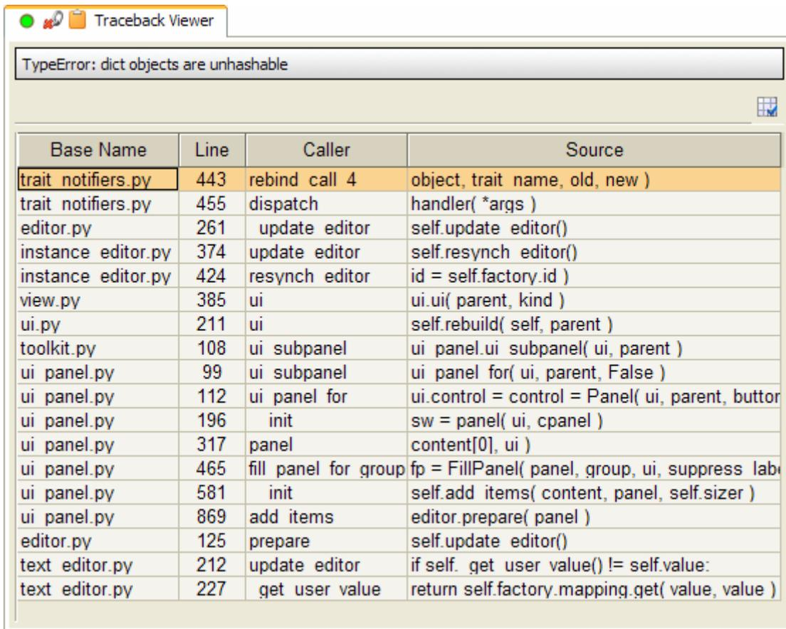
The message bar at the top of the view displays the exception that occurred, and the table below it shows the traceback entries for the exception, with one row for each stack frame, with the most recently executed stack frame at the bottom of the table.
