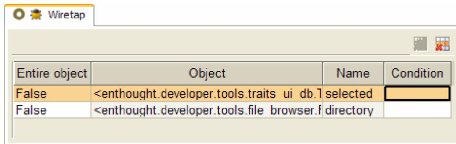
To create a wiretap breakpoint, drag a trait value from a tool such as the Universal Inspector and drop it on the Wiretap tool's drop icon (📍). Each time the specified trait changes value, the FBI debugger opens, displaying the source code line that changed the trait value.
